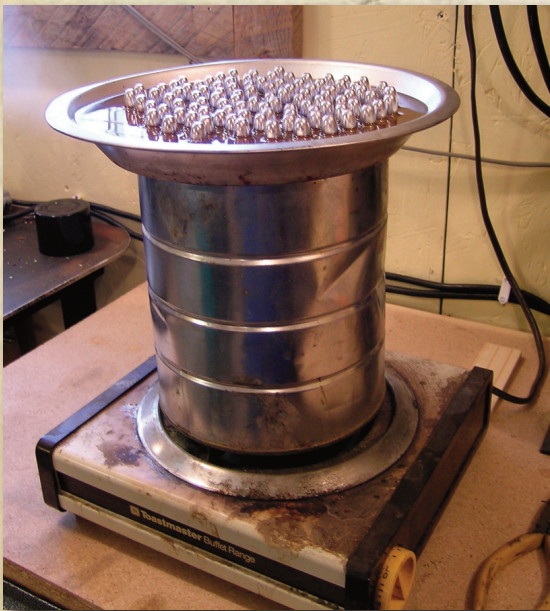
Double boiler utilizing a coffee can as the "water can". Pie tin holds melted lubricant and bullets.
